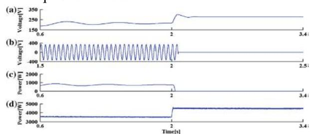
Figure 8. Matlab simulink outputs for transition from mode 2 to mode 3. a DC bus voltage. b Voltage of the grid. c Power delivered by the grid. d Power delivered by the PV array
