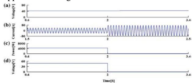
Figure 7. Matlab simulink outputs for transition from mode-1 case-2. a DC bus voltage. b Current flowing from the distribution transformer to the loads and the PEV. c Power delivered to the PEV (charging power). d Output voltage of the DC/DC buck converter
