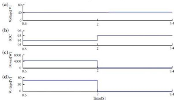
Figure 10. Matlab simulink outputs for transition in state-of-charge during mode-1. a DC bus voltage. b State-of-charge of the PHEV battery. c Charging power delivered to the PHEV. d Output voltage of the DC/DC buck converter
