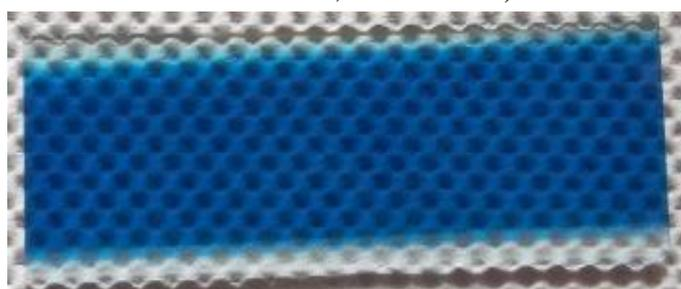
**Fig. 2. Phthalocyanine thin film on glass substrate**
