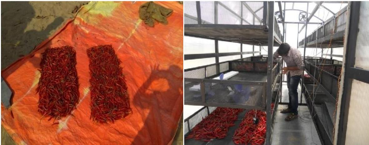
**Fig. 2. Different bed thickness in open sun drying and forced ventilated solar green house dryer.**
