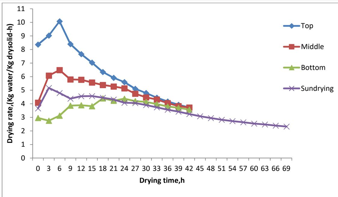
**Fig. 6. Variation of drying rates with drying time**
