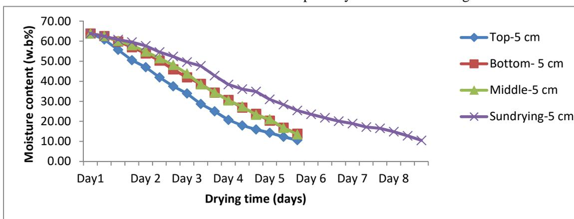
**Fig.5. Variation of moisture content of bed thickness 5 cm with drying time**
