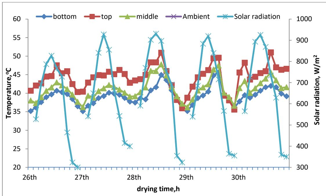
**Figure 3. Variation of different temperatures and solar radiation with drying time.**
