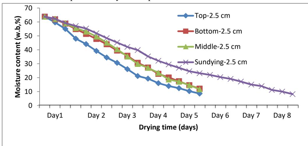
**Fig. 4. Variation of moisture content of bed thickness 2.5 cm with drying time**
