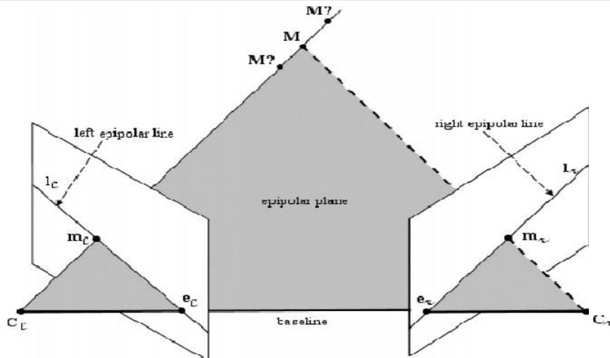
**Fig 2: Epipolar geometry**
