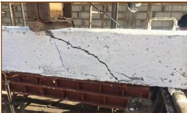
**Figure Failure Pattern of Beam**
