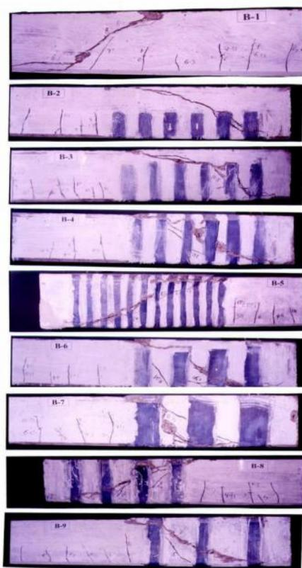
Fig : Crack patterns of tested beams.
