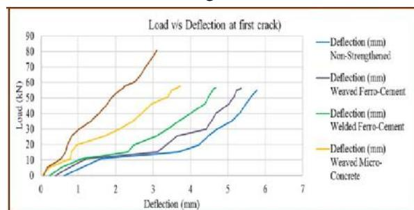
Fig : Load v/s Deflection at First crack
