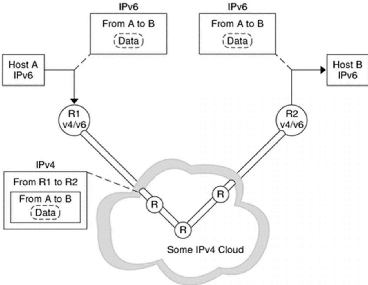
Figure -2 Tunneling mechanism
