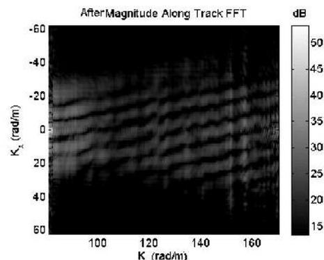
Fig4: Magnitude Response of Synthetic aperture position before phase
