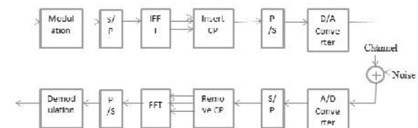
Fig1: Block diagram of OFDM Transmitter and Receiver model
