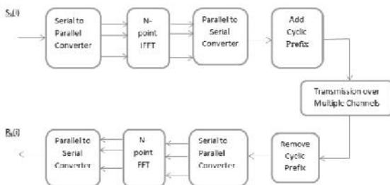
Fig2: Block diagram of OFDM system with prefix coding
