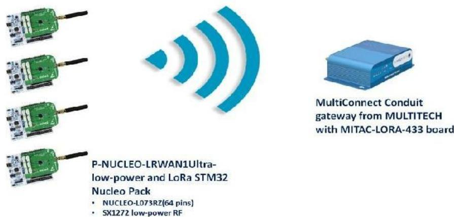
Figure 2: Example of End-node LoRa transceiver [13] and Gateway [14]
