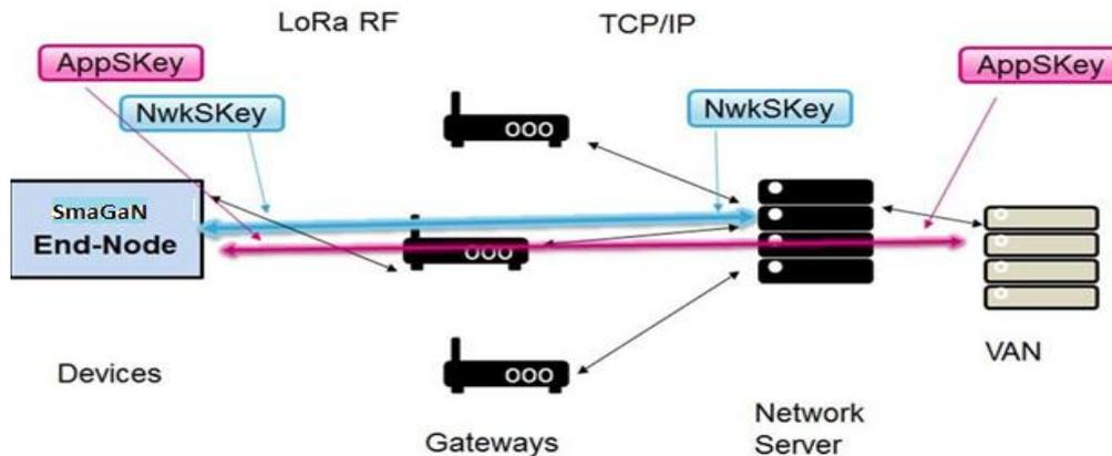
Figure 4: SmaGaN Security Design based on LoRaWAN
