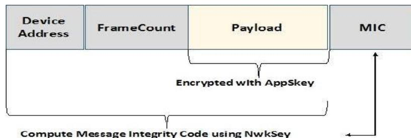
Figure 5: LoRaWAN Frame Format
