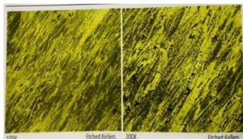
Fig 7: Optical Microscopic image of FSPed Al 7075
