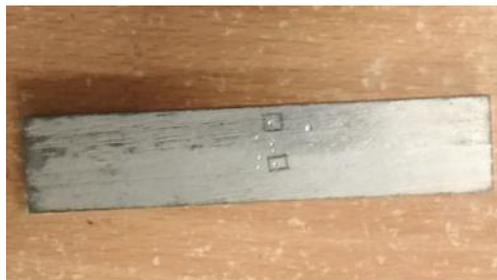
Fig 9(a) Rockwell Indentation upon Base metal
