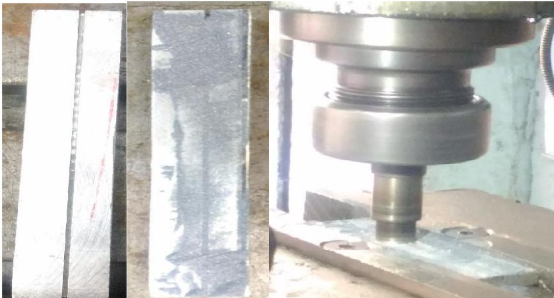
Fig 4 (a) & (b) Specimen before & after Filling of Silicon Carbide Powder
