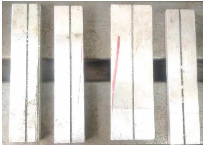
Fig 1: Base Metal Aluminium alloy Al7075
