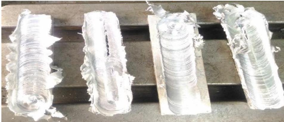
Fig.6 Surface of rotation speed at 1120 rpm and 1200 rpm
