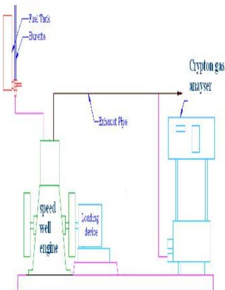
Fig.5 Experimental Set-Up
