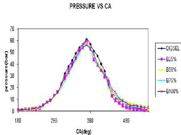
FIG 10.1 Peak Pressure with respect to Crank Angle
