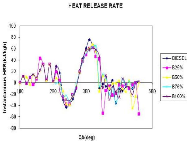
FIG 10.2 Variation of HRR with respect to Crank Angle
