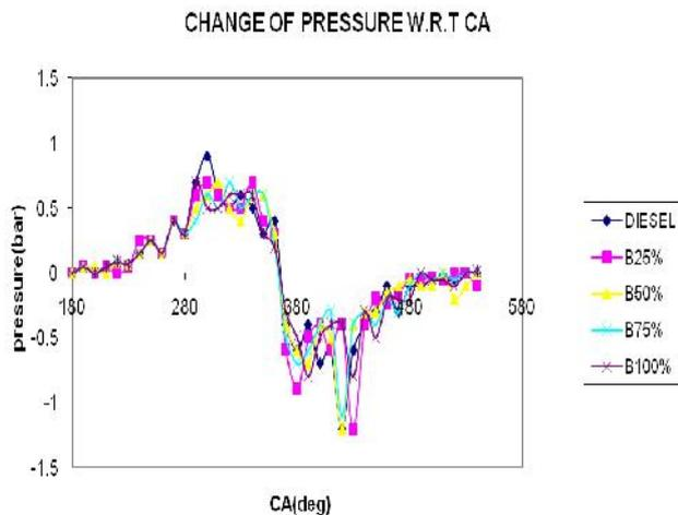
FIG 10.3 Change of Pressure with respect to Crank Angle
