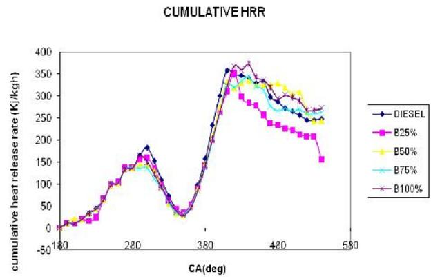
FIG 6.4 Variation of Cumulative Heat release Rate with respect to Crank Angle
