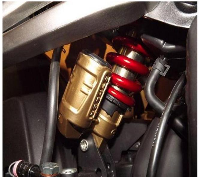
**Fig. 5. Nitrox Suspension [4]**
