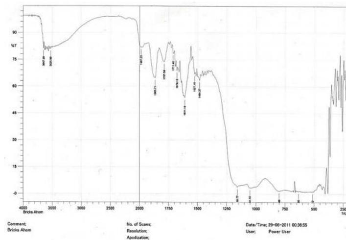
**Fig. 2 :** FTIR Spectra of Ahom Bricks
