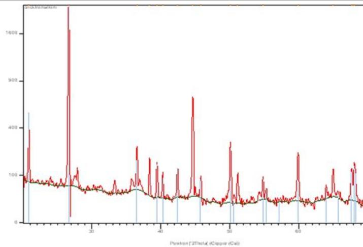
**Fig. 1.** XRD Spectra of the Ahom brick with copper target
