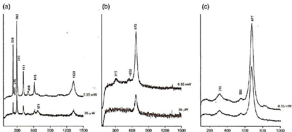
Figure 5(a): Raman Spectra corresponding to haematite (a) and magnetite (b & c)
