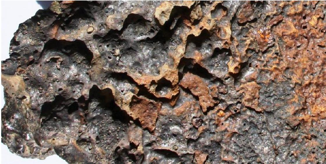
*Fig.2. a piece of lumpy iron slag collected from the area. The black shiny matrix is the physical characteristics that indicate the presence of silica; the reddish colour shows the probability of some iron contents. The big bubbles indicates that air has been blown to fire the ore minerals in the process of iron smelting and the air and water vapour trapped after the iron was extracted leaves these bubbles and vacuoles in the slag.*
