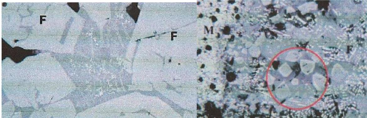
Figure (4- Left): Optical micrograph showing the transition from solid magnetite ore shows fayalitic slag (middle and right, marked as F).
