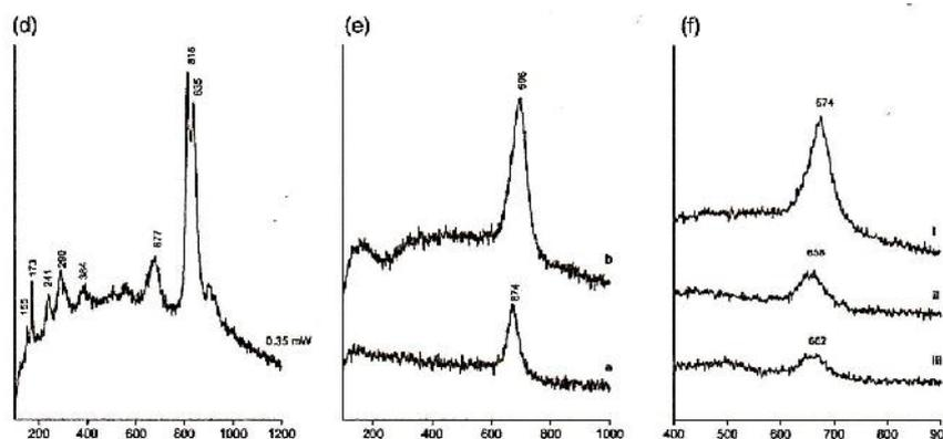
Figure 5(b): Raman Spectra corresponding to fayalite (d) and different compositions with fayalite matrix (e & f).
