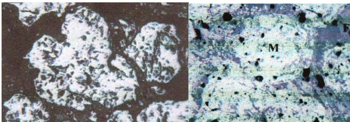
*Figure (3- Left): Optical micrograph of a piece of ore embedded in iron slag, mainly magnetite (darker crystals, marked M) and haematite (lighter lamellae, marked H). Black is open porosity and cracks run through this ore, possibly due to an earlier roasting stage.*
