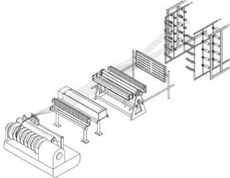
**Fig. 5 Warping system with plates**
