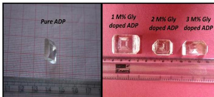
**Figure 1: Photographs of Grown Pure and Glycine Doped ADP Crystals**
