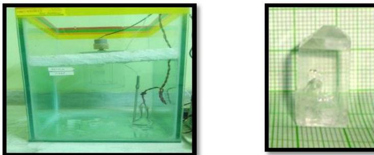
**Figure 2: Experimental Set-up of Rotation Method and Photograph of Grown Glycine Doped ADP Crystal**
