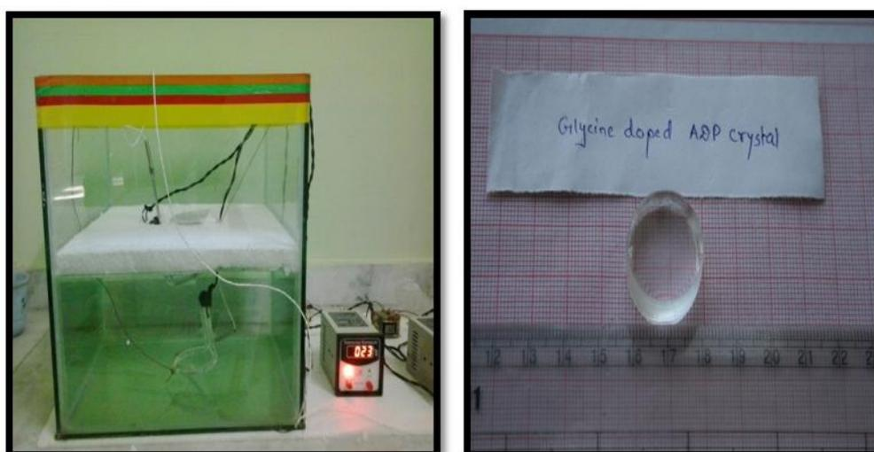
**Figure 3: Experimental Set-up for SR Method and Photograph of Glycine Doped ADP Crystal**
