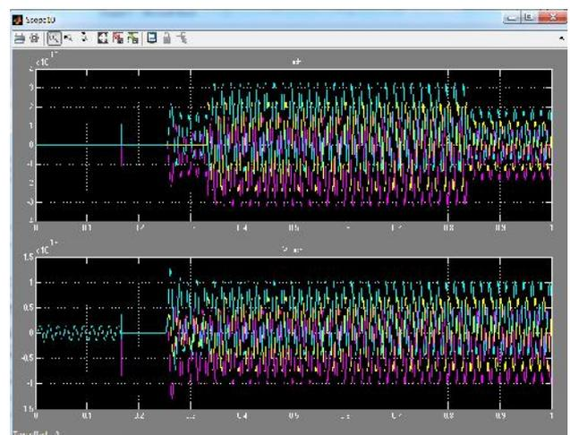
**Figure 14: (a) Three phase current waveform at bus six (b) Three phase voltage waveform at bus six with fault at bus five**
