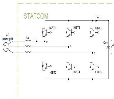
**Figure 3: Power circuit diagram of a STATCOM**
