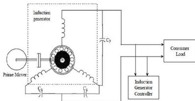
**Figure 1: Schematic diagram of Single phase SEIG [10]**
