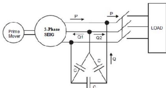
**Figure 2: Schematic diagram of three phase SEIG [11]**
