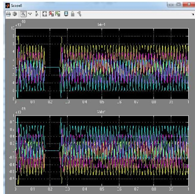
**Figure 13: (a) Three phase current waveform at bus no. seven (b) Three phase voltage waveform at bus number seven with fault in bus number five.**
