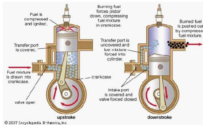
Fig:- 2-Stroke Engine
