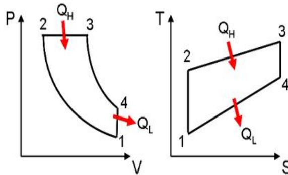
Fig:- P-V And T-S Diagram of Diesel cycle.
