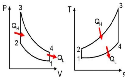
Fig:-P-V And T-S Diagram of Otto Cycle
