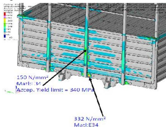
Fig.7 side pillar for bump condition
