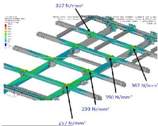
Fig.6 Cross member for cornering condition
