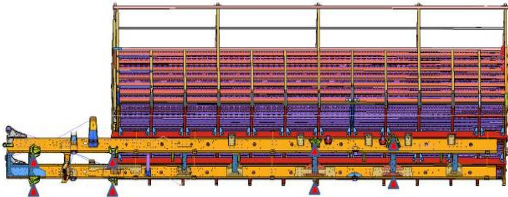
Fig 1 Model of Load body with its boundary condition
