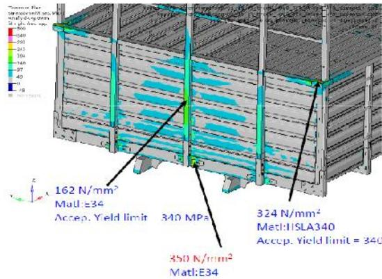
Fig.2 Side pillar for braking condition
