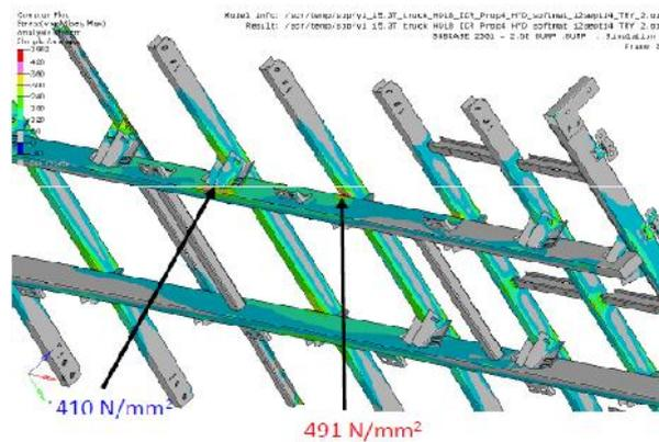
Fig.9 Sub frame for bump condition
