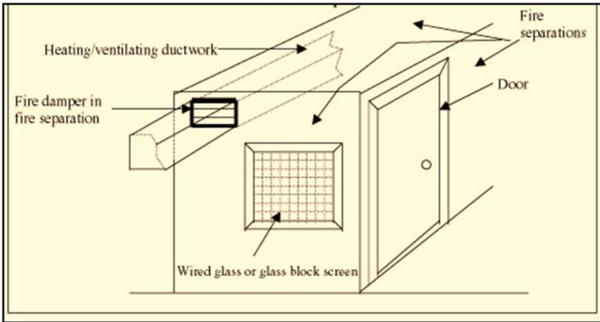
**Fig.6: CLOSURES IN FIRE SEPARATION**
