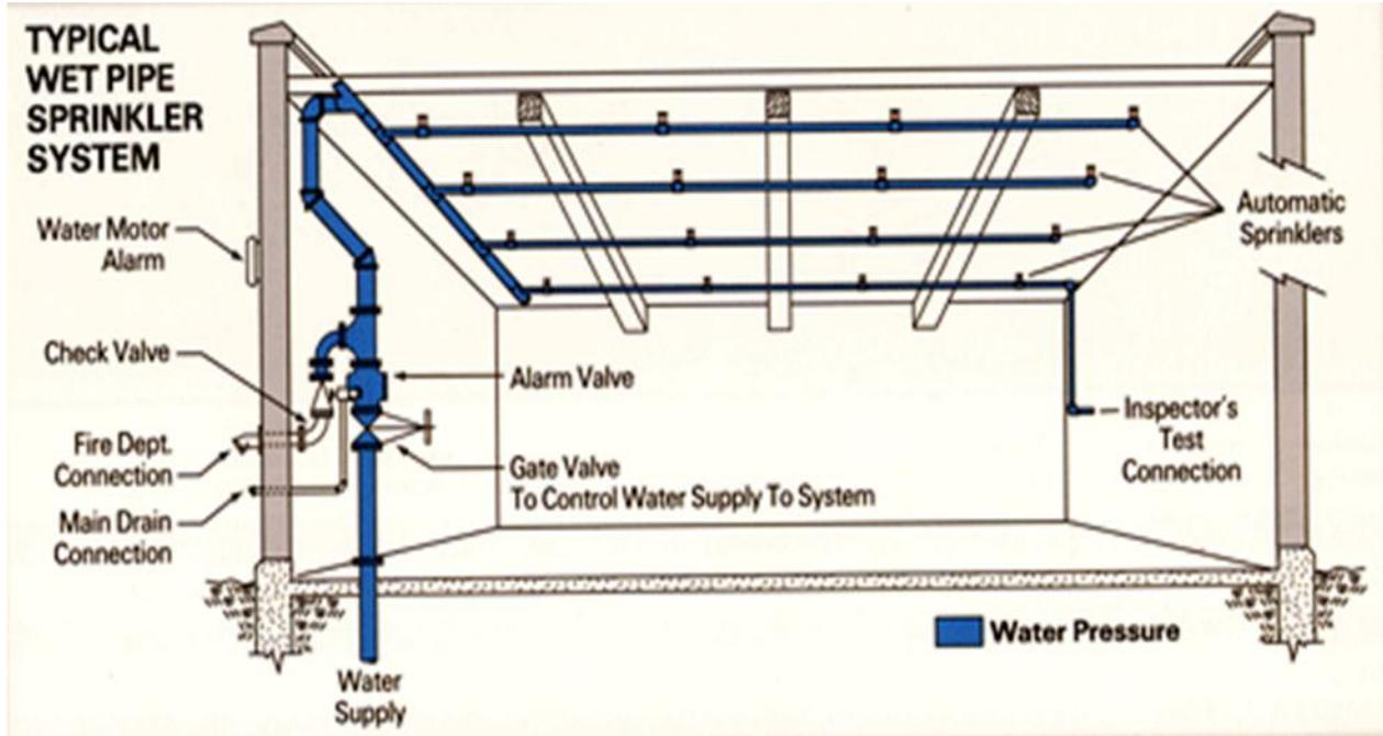
**Fig.16 WET PIPE SYSTEM**
