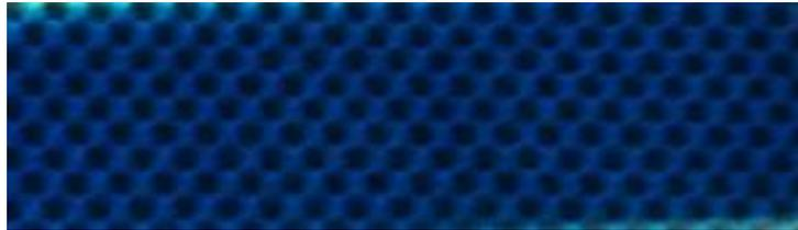
**Fig. 2. Phthalocyanine thin film on glass substrate**
