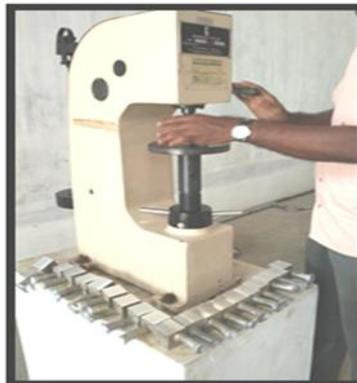
**Figure: 1 Brinell Hardness Tester (BHN)**
