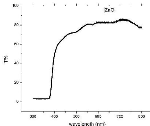
**Fig 2: Optical transmittance spectra of ZnO**
