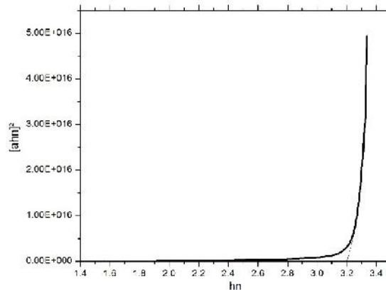
**Fig 4: Tauc's plot obtained from UV-Vis transmittance spectra of ZnO thin film**
