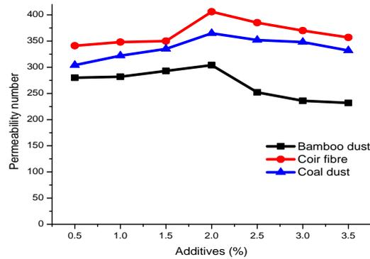
Fig. 1 Variations of additives vs Permeability number
