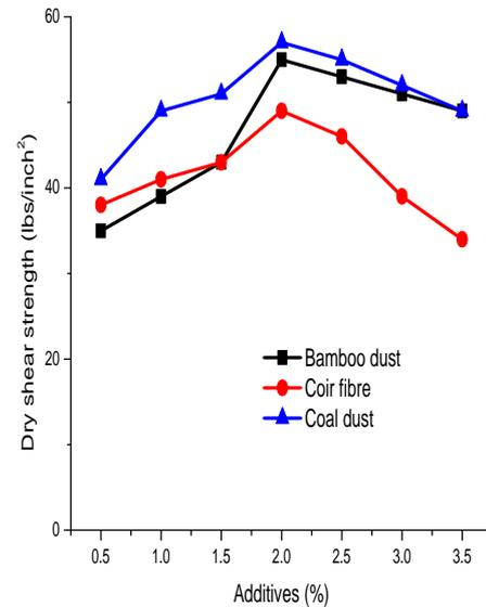
Fig. 5 Variations of additives vs Dry shear strength
