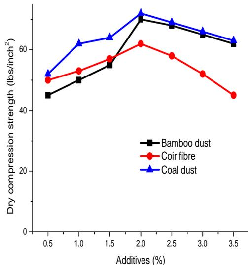
Fig. 4 Variations of additives vs Dry comp. strength
