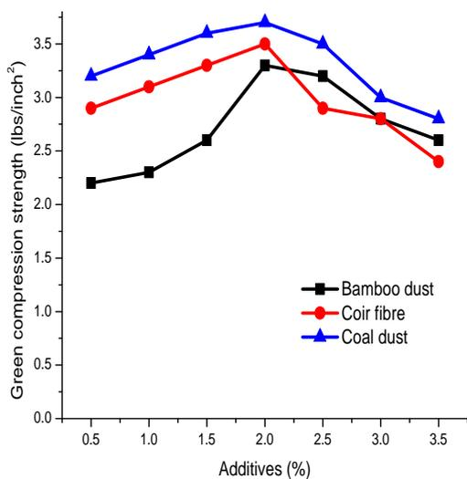
Fig. 2 Variations of additives vs Green comp. strength
