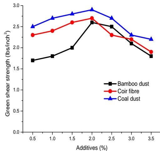
Fig. 3 Variations of additives vs Green shear strength
