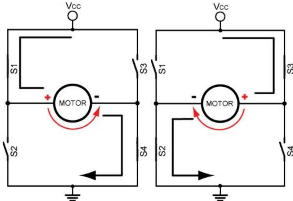
**Fig 2: motor runs in clockwise (switches 1 and 4 closed)**
