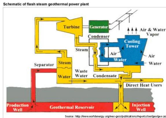
**Figure5:Block Diagram of Electricity Generation by Geothermal**
