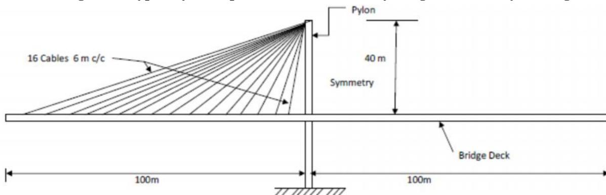
**Fig. 3 Details of fan type stay cable profiles used in manually design**
