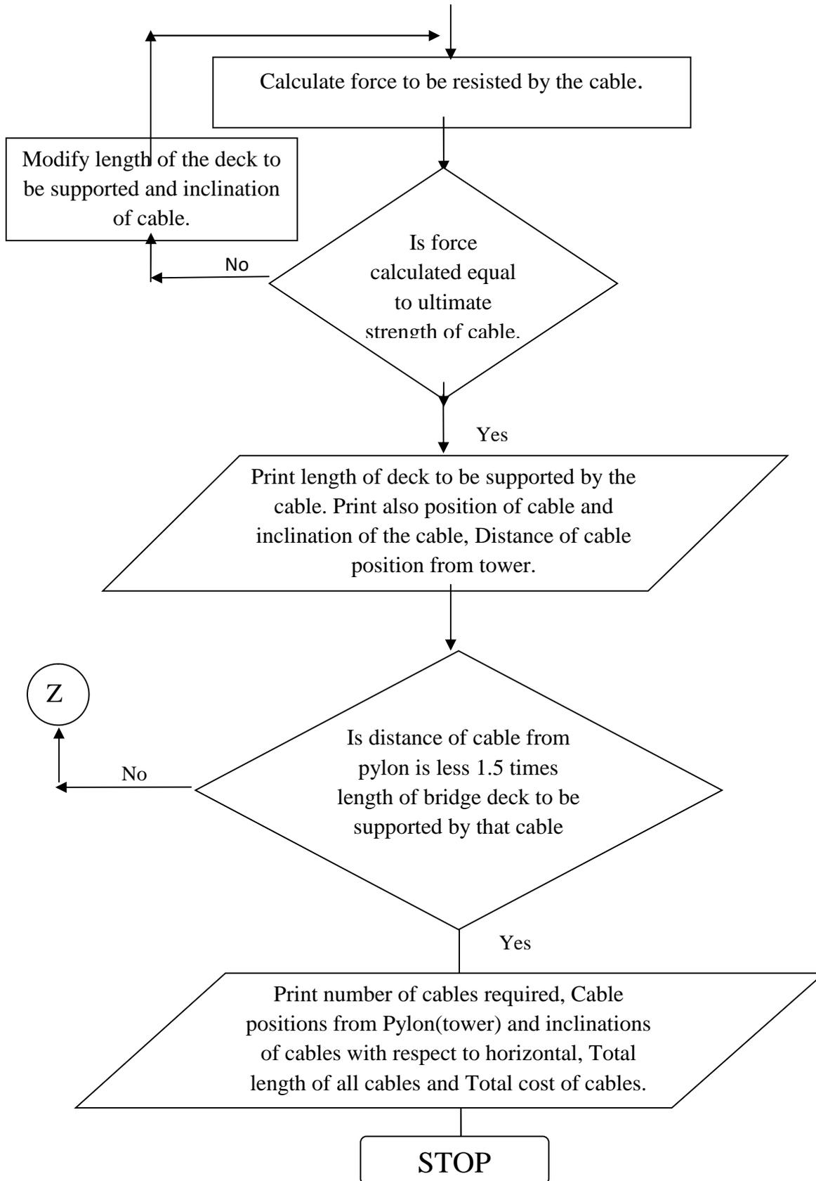
**Fig.1 A flow chart for optimum design of fan type stay cable profiles**
