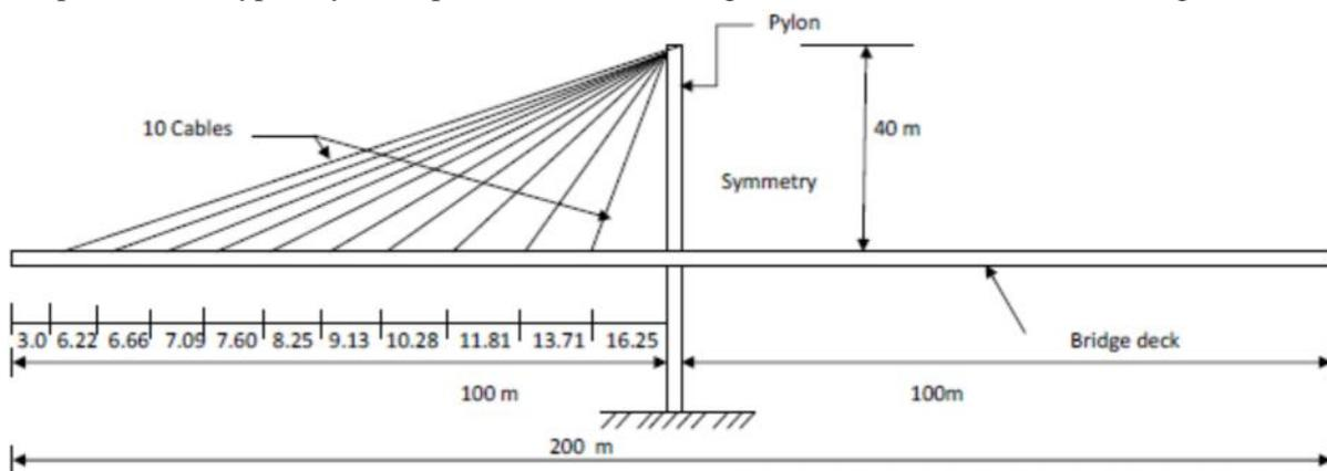
**Fig. 4. Optimized fan type stay cable profiles for the problem shown for one Pylon(Tower).**
