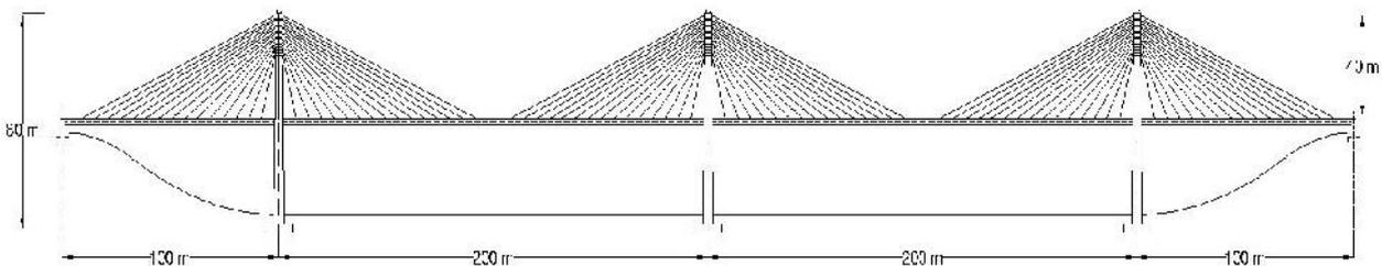
**Fig 2. Fan type stay cable profiles used in manually design of cable stayed bridge**
