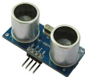
**Figure 3: Ultrasonic Sensor**
