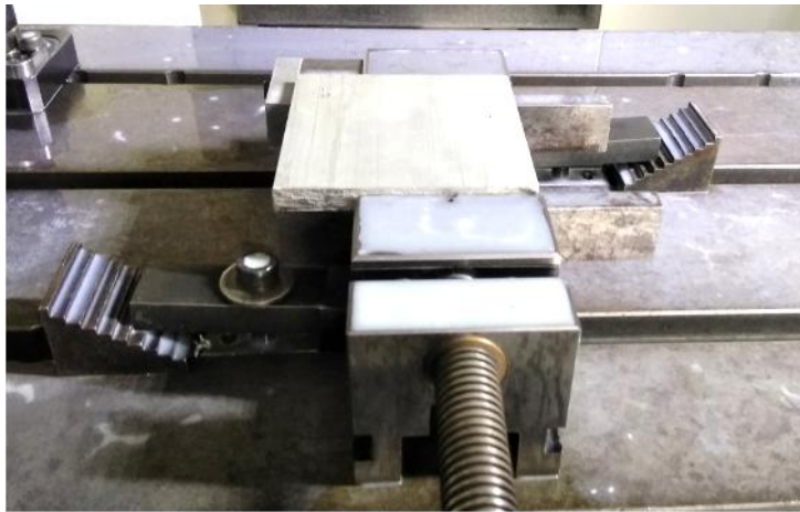
Fig 11: Holding Fixtures applied to Aluminium Plate
