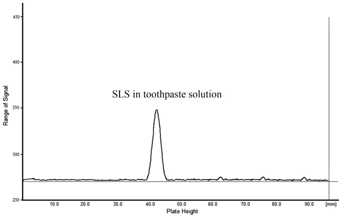
**Figure 3:** Densitographic representation of SLS identified in toothpaste solution.
