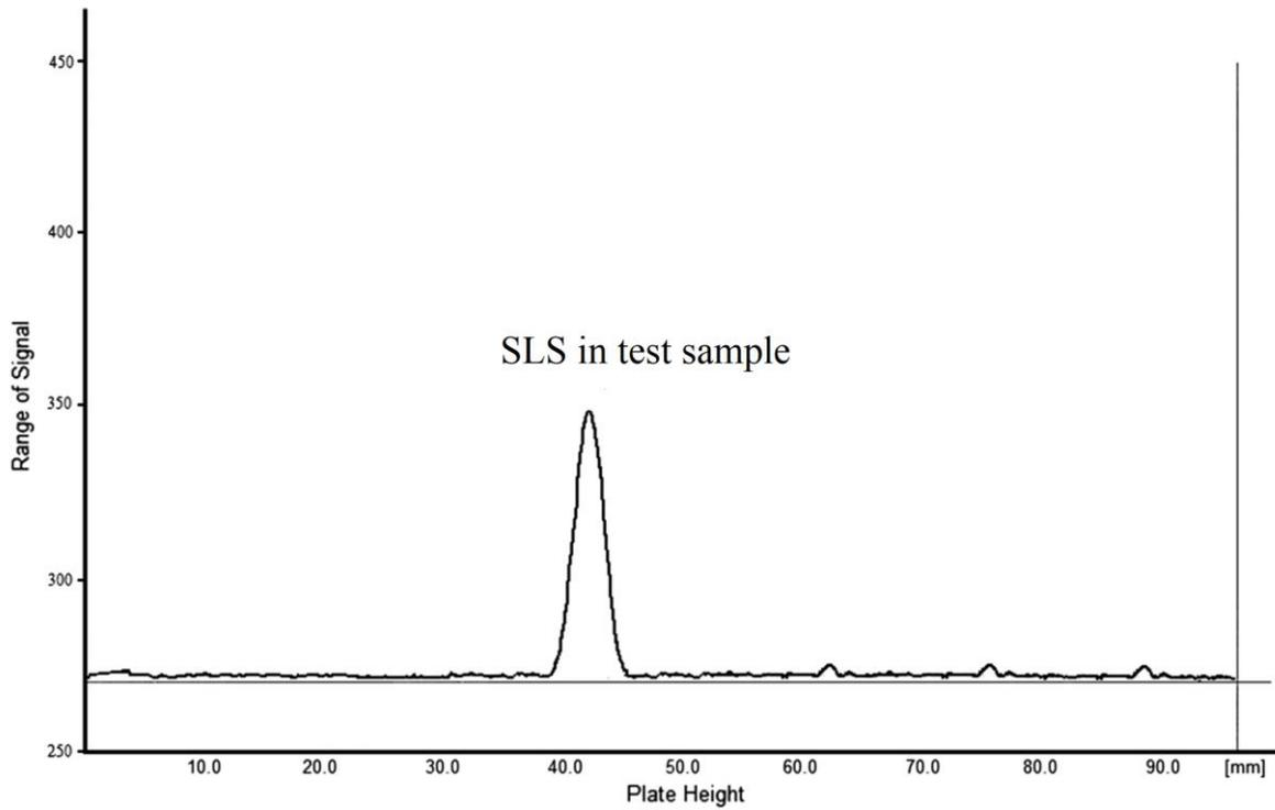
**Figure 2:** Densitogram of SLS in test solution.
