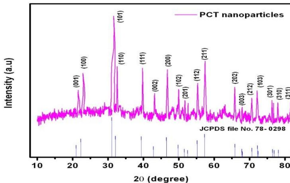
**Fig.1. XRD pattern of PCT nanoparticles**
