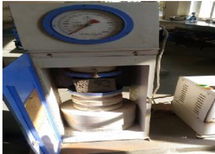
Fig1. Cube testing by compression testing machine
