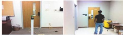
Fig 11: UWB RADAR and human target for wooden door.
