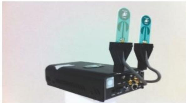
Fig 7:UWB P220 in monostatic mode<sup>[2]</sup>.
