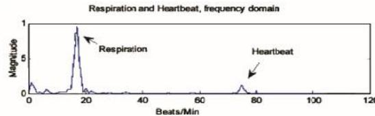
Fig 6: The waveform of heartbeats and respiration in frequency domain.
