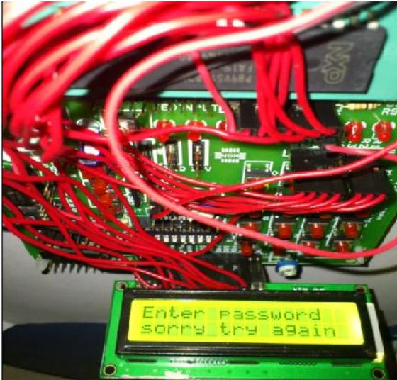
**Fig 3: Output when wrong password entered**
