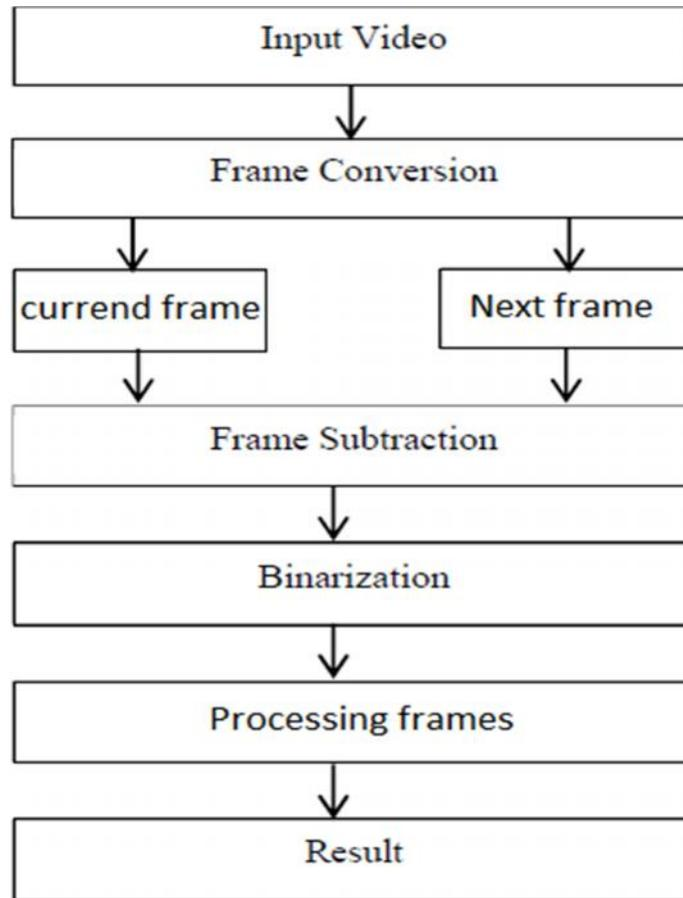
**Fig. 2: Flow chart of frame processing**
