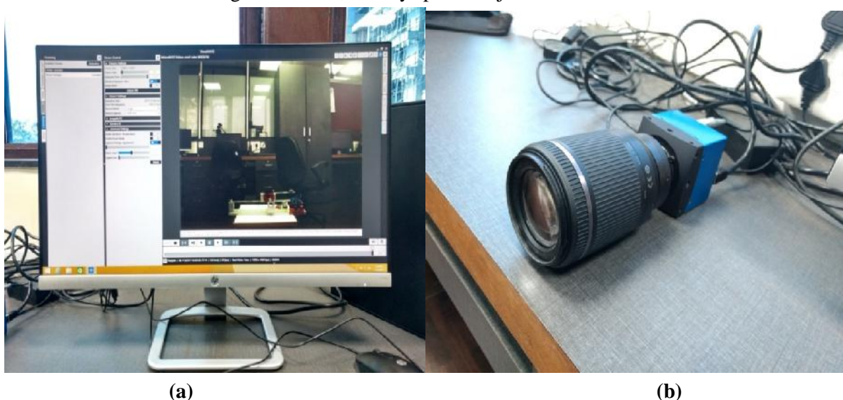
Fig. 1 Computer with VisualiMarc (software for video capturing) and Visual studio/OpenCV for algorithm implementation(a), Mikrotron high speed camera with extended lens(b)
