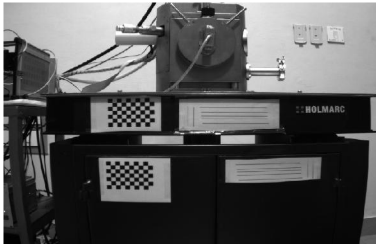
Fig. 2 Scanning electron microscope platform with checkbox artificial template.
