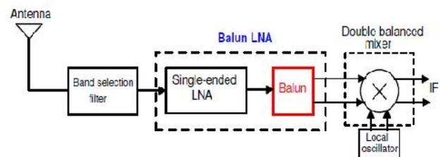
**Fig.1: Receiver with balun LNA (reproduced from [2])**
