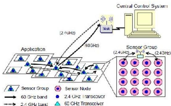
**Fig.2: Hierarchical architecture of WSN system (reproduced from [3])**
