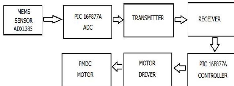
Fig.1 Block diagram of implemented control
