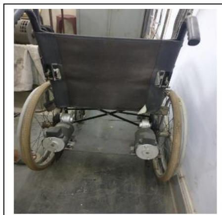
Fig.3 Wheelchair fitted with motors
