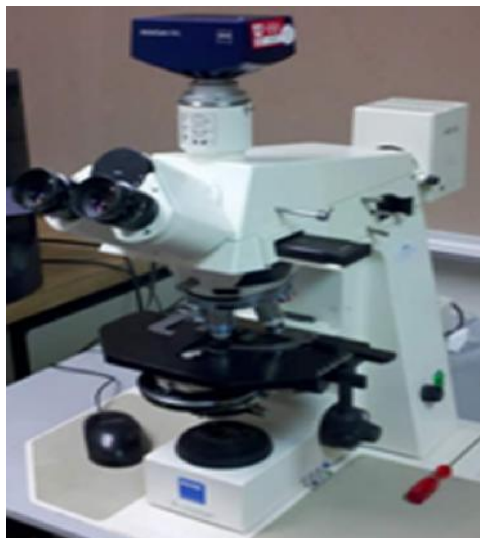
Fig 4. Zeiss Optical Microscope: Microscopic Optical Examinations of Post-Test Filament Specimens.
