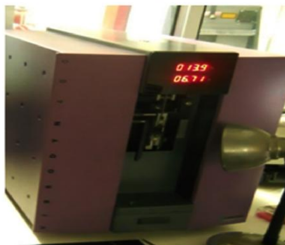
Fig 2. Vibrodyng Machine: Determination of the Tensile Strength of the Filament.
