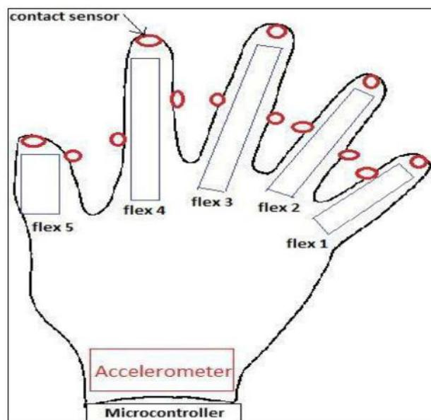
**Fig3: Labeling of sensors on the glove**
