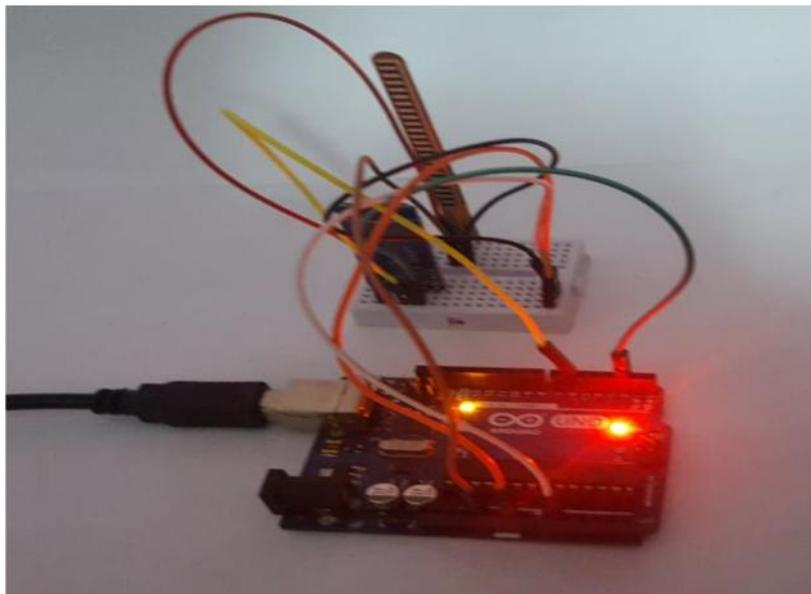
**Fig 4:Initial implemented circuit consisting of flex sensors and Bluetooth module**
