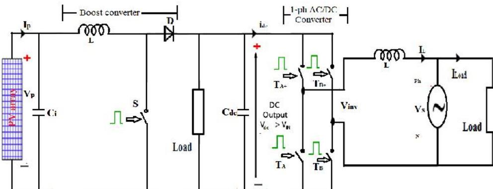
**Fig 2: Circuit diagram of the proposed grid-connected PV system**
