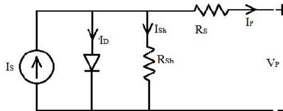
**Fig 3: Equivalent of the PV panel**
