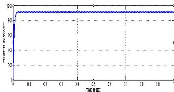
**Fig 7: Simulation results of PV array power with Fuzzy based MPPT controller**
