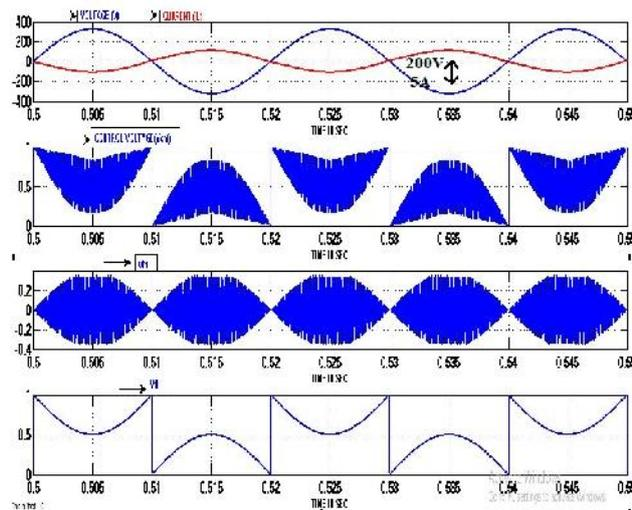
Fig 12: Simulation results with pure sinusoidal AC grid voltage: Grid voltage and line current, control signal, feedback signal and feedforward signal when converter operated in inverter mode using feedforward control
