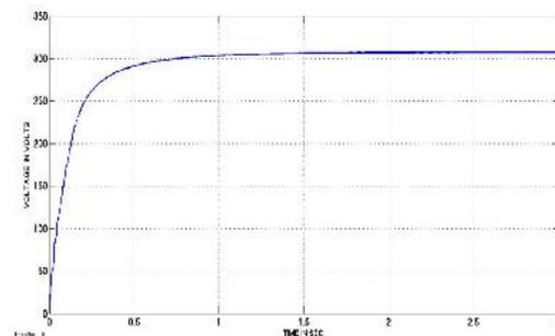
**Fig 8: Simulation results of the boost converter output voltage**
