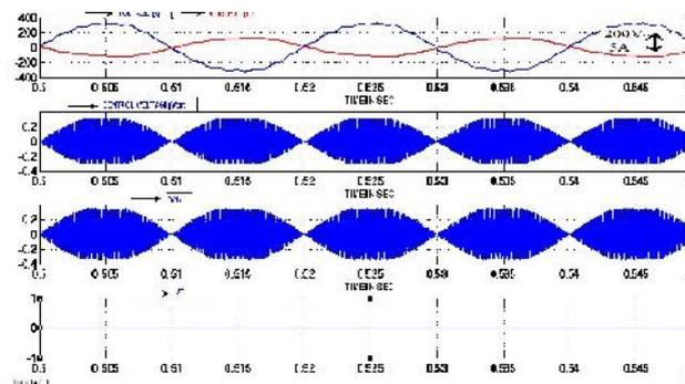
**Fig 16: Simulation results with distorted AC grid voltage: Grid voltage and line current, control signal, feedback signal and feedforward signal when converter operated in inverter mode using conventional control**
