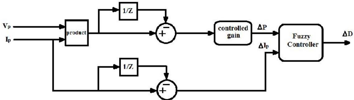
**Fig 5: Block diagram of the Fuzzy based MPPT controller**
