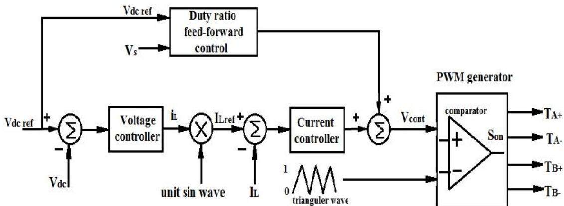
**Fig 10: Conventional control scheme for single-phase bidirectional AC/DC converter**
