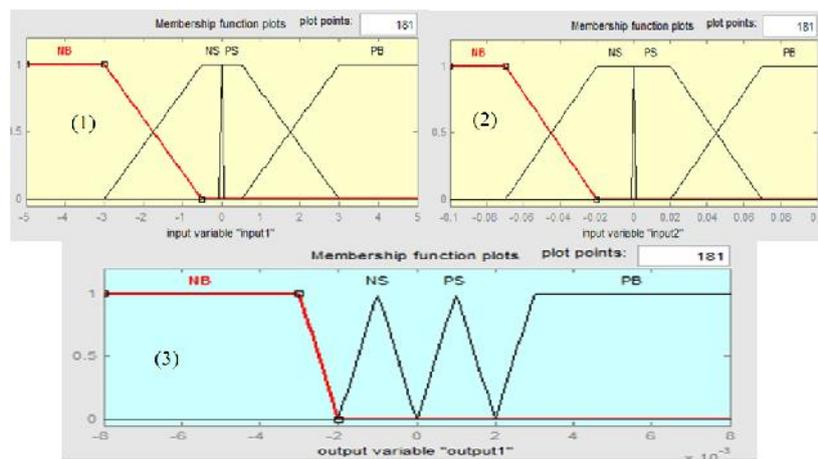
**Fig 6: Input (1)(2) and Output(3) membership functions of fuzzy controller**
