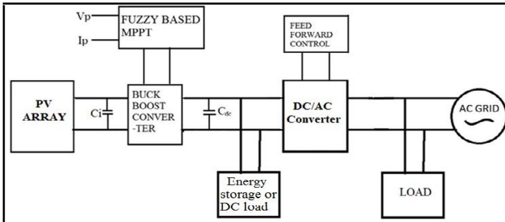
**Fig 1: Schematic block diagram of the grid tied PV system**
