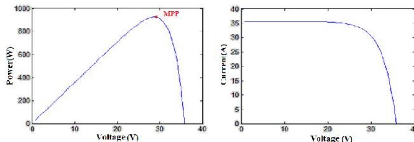
**Fig 4: P-V & I-V characteristics of 1kW PV array**
