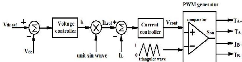
**Fig. 9: Conventional control scheme for single-phase bidirectional AC/DC converter**
