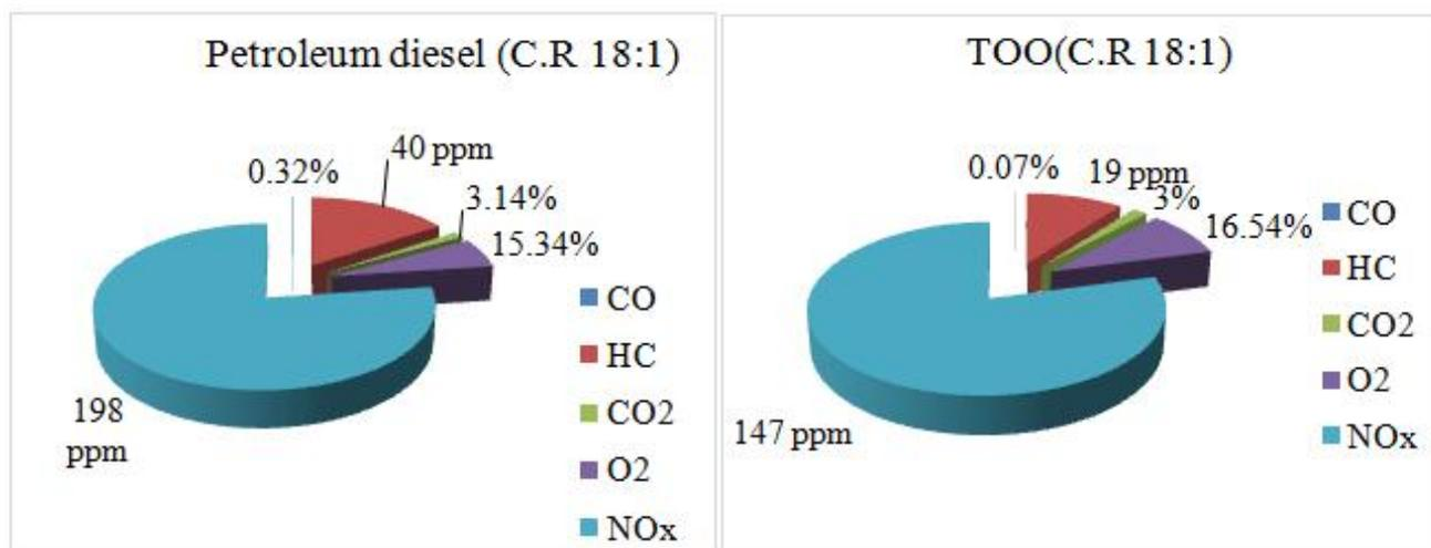
Fig. 11 Emission comparison of TOO with petroleum diesel
