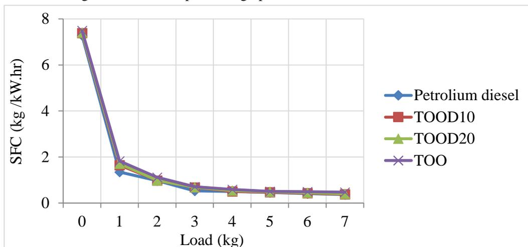
Fig. 8 Variation of specific fuel consumption with load
