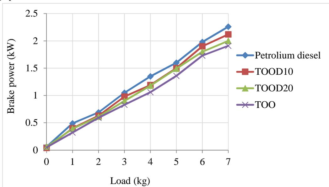
Fig. 5 Variation of brake power with load
