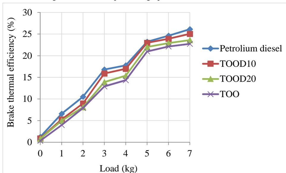
Fig. 7 Variation of brake thermal efficiency with load
