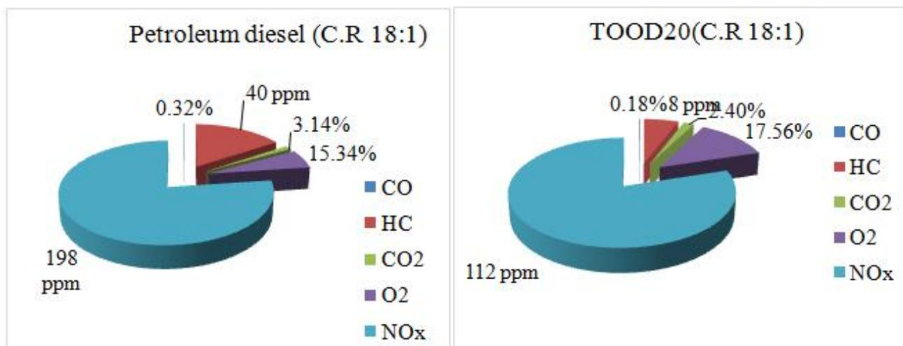
Fig. 10 Emission comparison of TOOD20 with petroleum diesel
