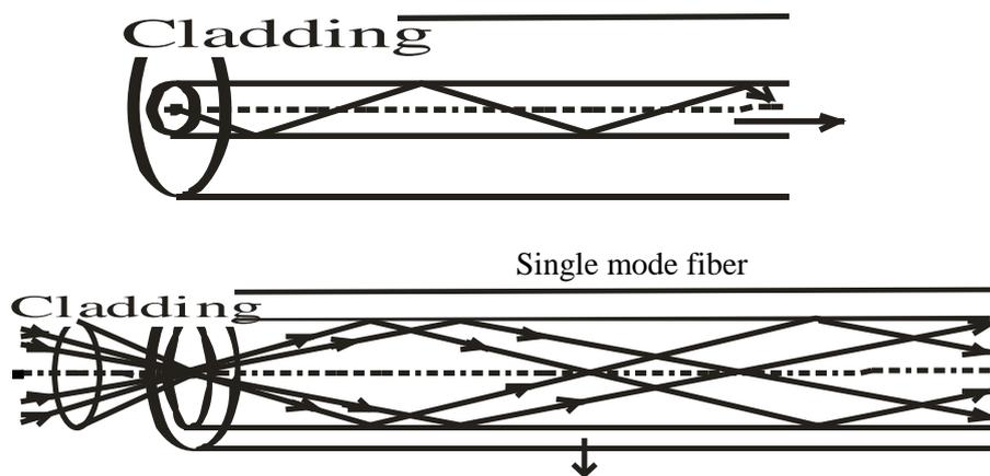
Figure 2. Single mode and Multi mode fiber
