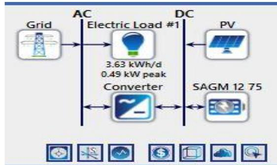
Fig 1: Simulation of test case
