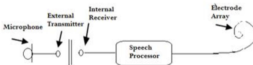
**Fig 1 : Implantable system of a transcutaneous cochlear implant.[1]**
