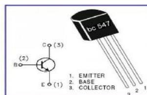
**Fig 3.5 Transistor**
