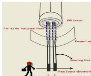
**Fig 3.2: Pin configuration of PIR sensor**
