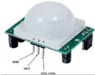
**Fig 3.1: Passive Infrared Sensor (PIR)**
