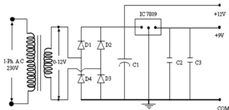
Fig.8 CIRCUIT DIAGRAM OF POWER SUPPLY UNIT
