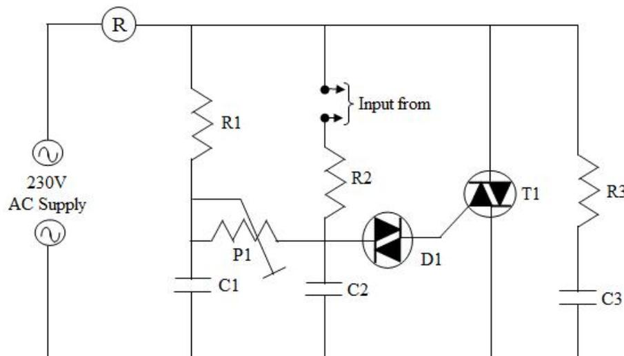
**FIG.7 CIRCUIT DIAGRAM OR FAN DRIVER SECTION**
