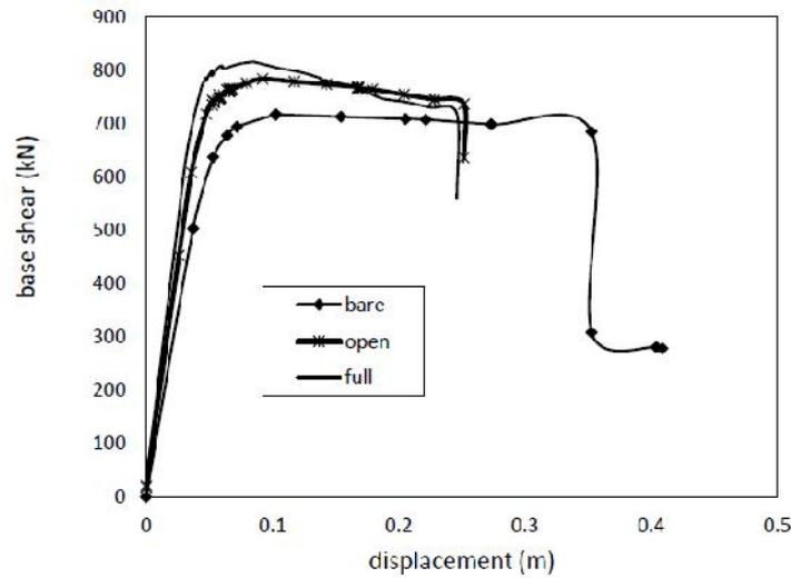
**Fig. 7: Comparative Pushover Graph Between The Rectangular Building With Different Infill Cases**
