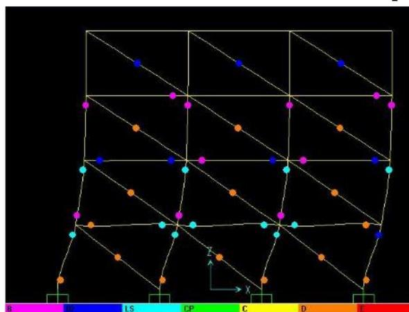
**Fig. 6 Hinge Formation For Frame With Full Infill**
