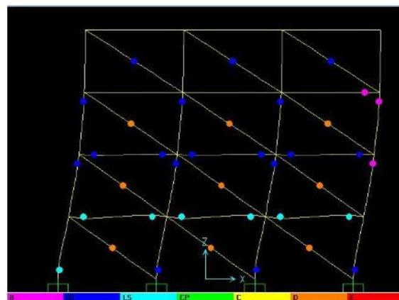
**Fig. 9 Hinge Formation For Frame With 25% Of Openings In Infill**
