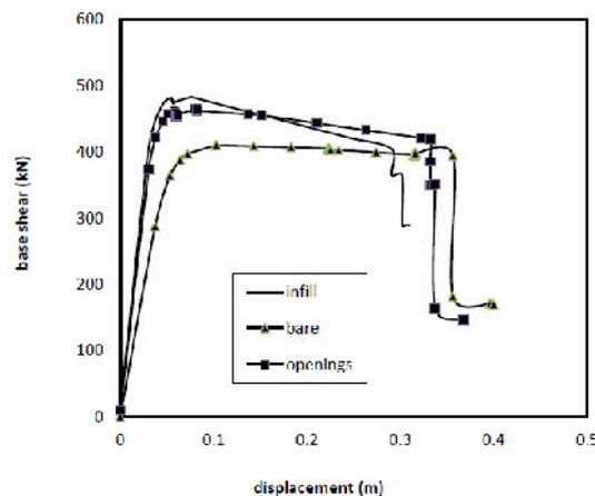
**Fig. 3: Comparative Pushover Graph Between The Square Building With Different Infill Cases**
