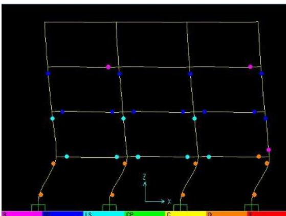
**Fig. 8 : Hinge Formation For Bare Frame**
