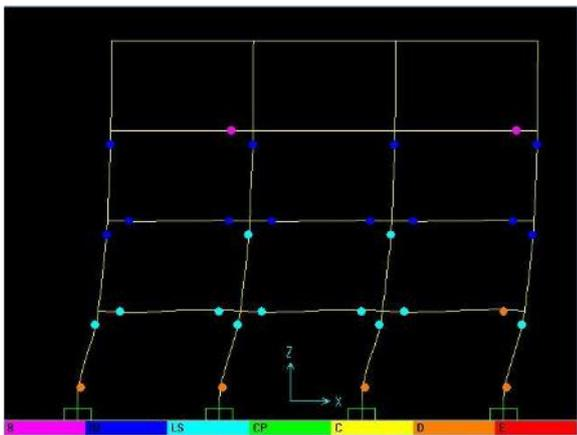
**Fig. 4 : Hinge Formation For Bare Frame**
