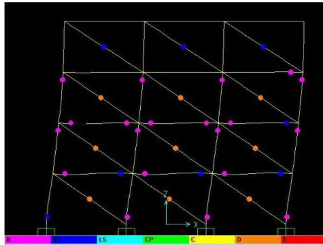
**Fig. 10 Hinge Formation For Frame With Full Infill**
