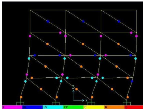
**Fig. 5 Hinge Formation For Frame With 25% Of Openings In Infill**
