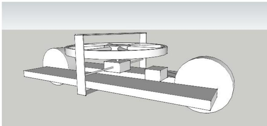
**Fig 5:**Isometric view of the two wheeler in 3D (Isometric View)
