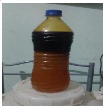
**Figure 5: Top bio-oil and bottom viscous liquid layers**
