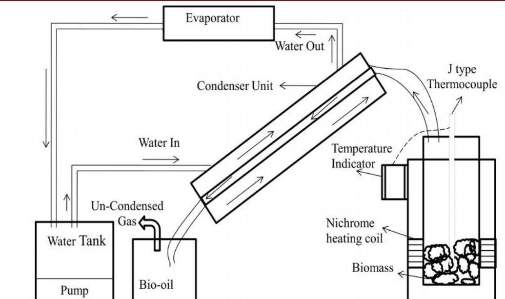
Figure 3: Experimental setup
