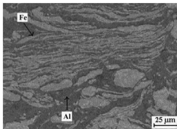
**Fig1: Microstructure of Fe-Al Mechanical Alloy captured by Scanning Electron Microscope**
