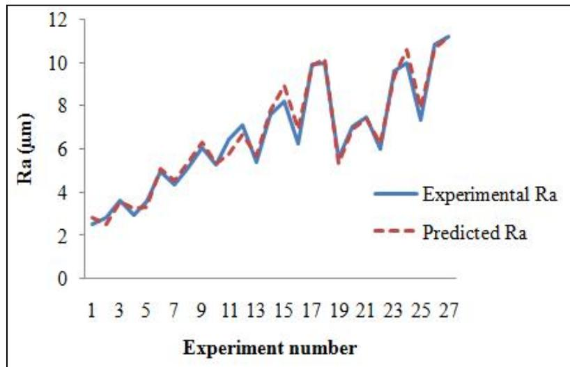
**Fig 7: Comparison of experimental and analytical surface roughness values**
